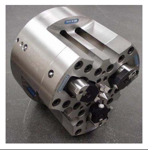
Powerhold Retractable Jaw chucks are a 2-in-1 chuck that combines a 3-jaw power chuck and face driver into one assembly. When turning shafts or gun barrels, accuracy often demands turning the entire length in a single operation. Face driving alone requires a lighter cut and long cycle times. The retractable jaw chuck, or shaft-chuck, solves this problem.
